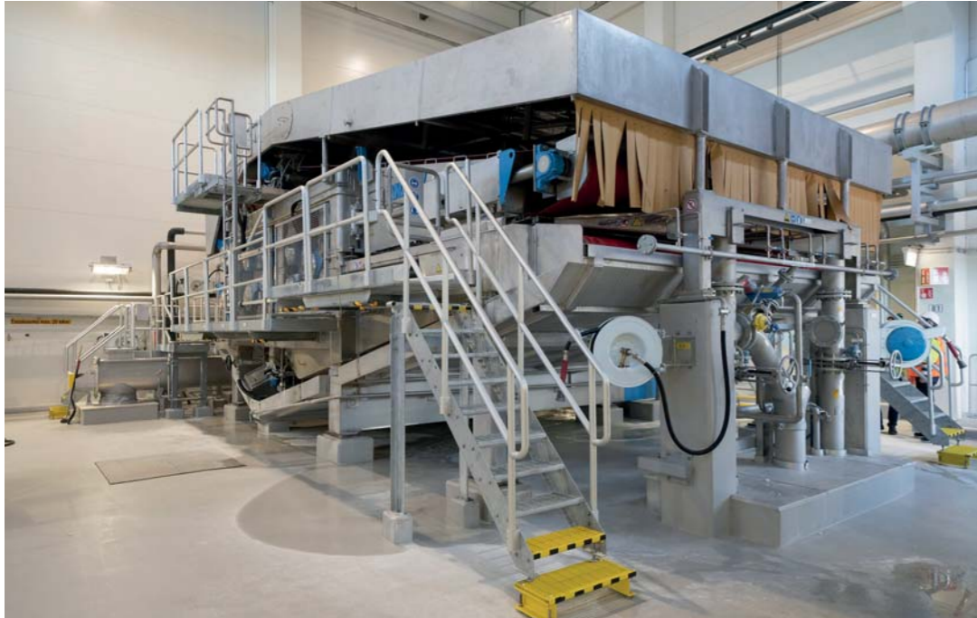
The ANDRITZ Twin Wire Press has been proven in many applications for all pulp types and is the best suited thickening equipment prior to a Flash Dryer
