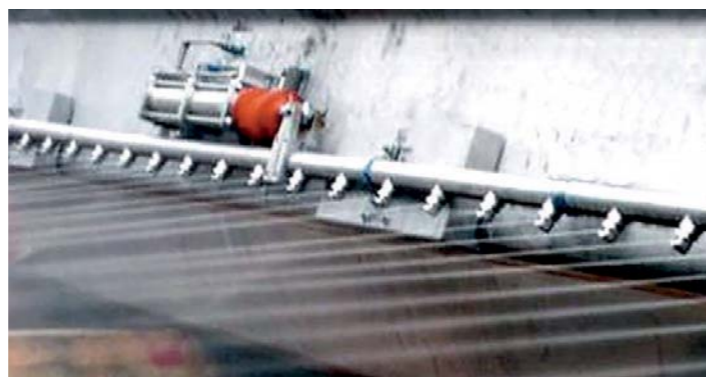
Roll upgrades Valmet Suction Roll Upgrade Shell Flow H: Suction roll hole cleaning system for enhanced dewatering.
