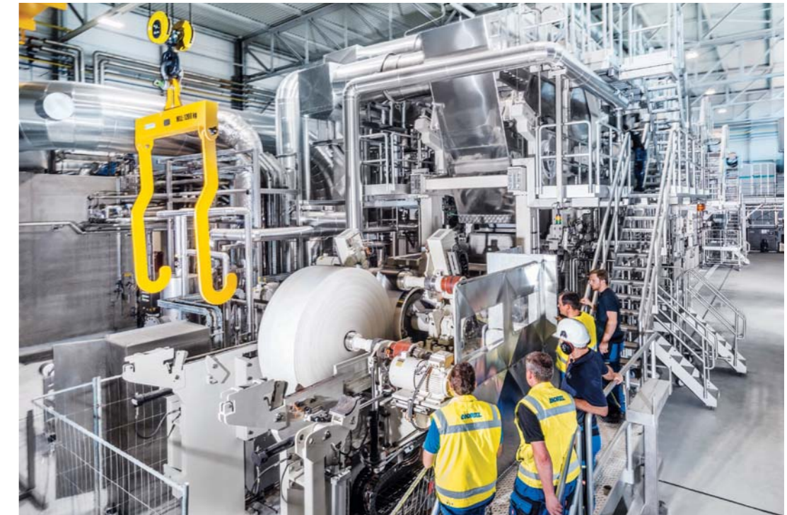
The Innovation and Application Center (PrimeLineTIAC) features a tissue pilot plant for the production of dry-crepe, structured, and textured tissue
