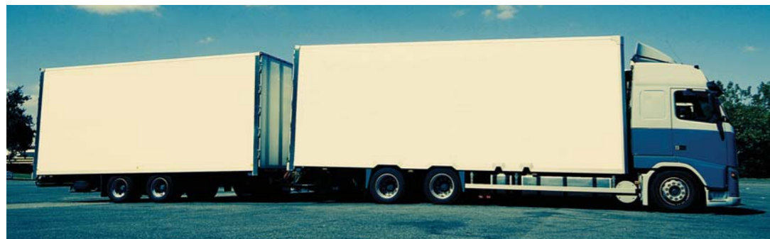
Megatrucks could result in up to 25 per cent fuel savings
