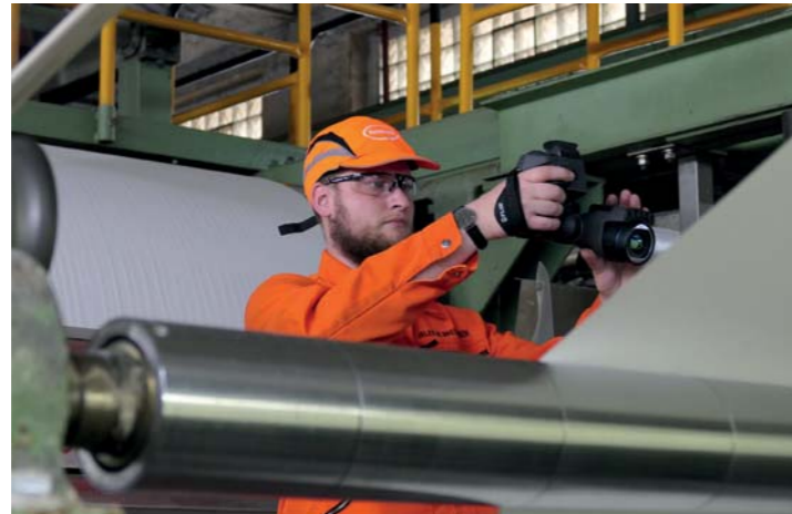
One of Heimbach's TASK team carries out a thermographic measure on a paper making line
