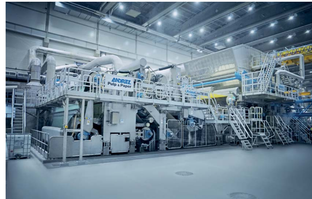
Arkhbum's new tissue machine is running at 2,000 m/min
