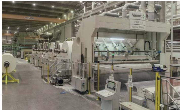
A rewriter is the toolbox that enables the tissue machine output to satisfy every consumer's need
