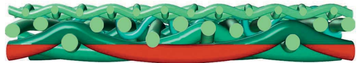
Figure 2: Premium solution: Eight-shaft weave pattern on the machine side
